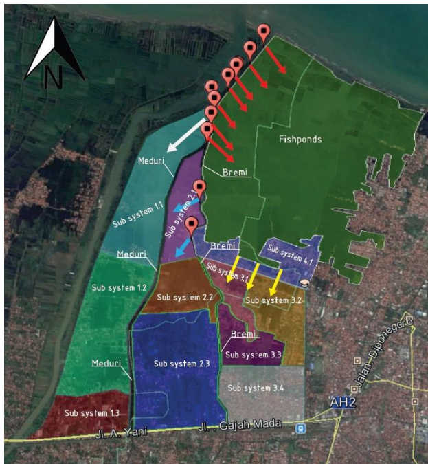
Figure 6, red dots show the locations where sea water intrudes the fishponds during high tide. The red arrows illustrate the connections with the fishponds. The white arrow with sub system 1.1, the blue arrows with sub system 2.1 and the yellow arrow with sub system 4.1.
