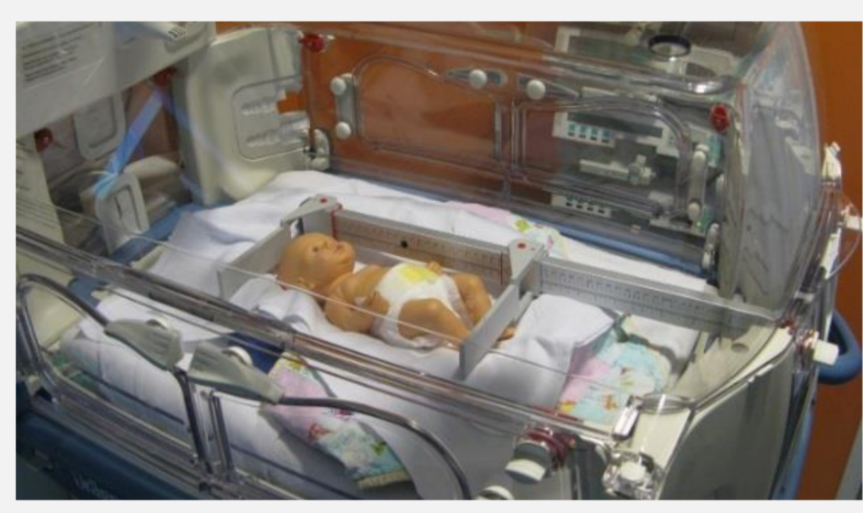
Current instrument (slide calliper) for length-measurement of a premature infant inside an incubator: big, clumsy, unhygienic and very stressful for the infant.
